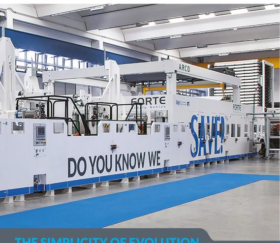
The simplicity of the concept it is based on allows **FORTE** to continually enhance its performance and to evolve, providing the market with an incomparable finished product. The key to **FORTE**'s success are three winding rolls cleverly positioned and moving in relation to one another, generating soft, perfectly wound toilet rolls and kitchen towels at high speed, guaranteeing a total quality finished product. And all using a minimal technology, simple to use and reliable in time.
