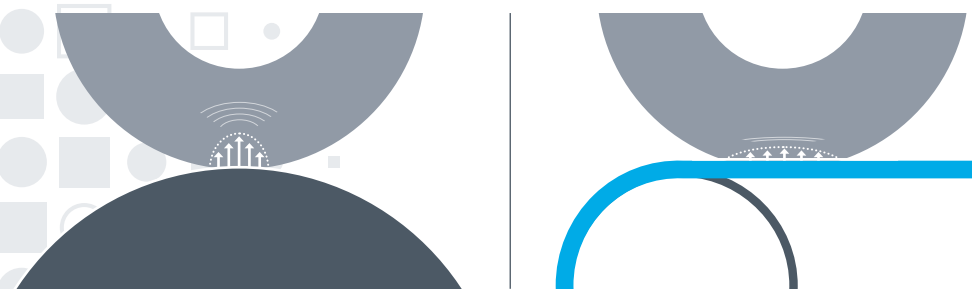
PARAGON's increased contact area at the same force reduces nip pressure and avoids caliper crushing.
